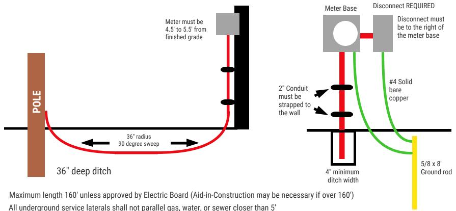
A minimum of 5' of clearance must be provided between electric metering equipment and gas unless approved by Electric Board personnel
